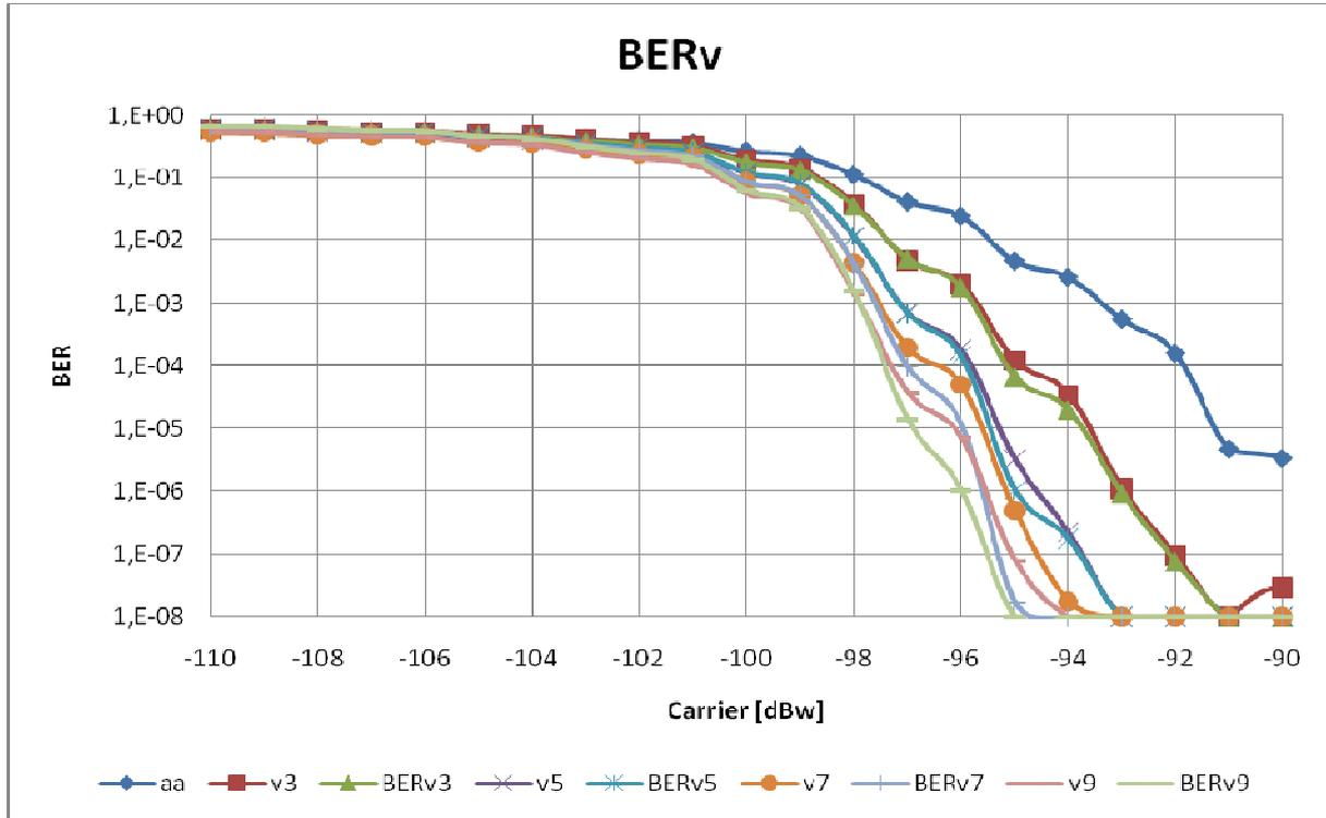
**Fig 9. Comparison of a voted algorithm improving radio link quality depending on the number of receivers.**
