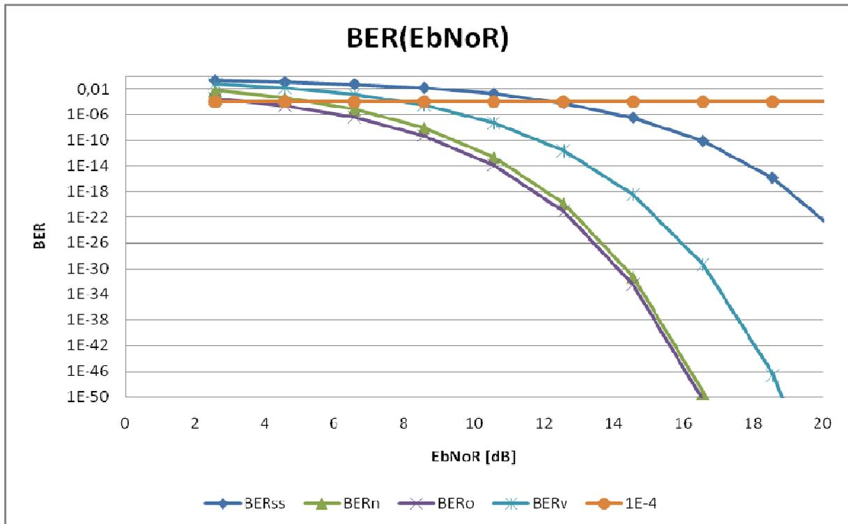
**Fig 5. BER depending on EbNoR in a single station link balance.**
