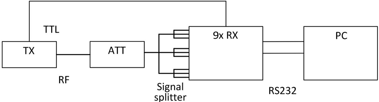
**Fig 6. Diagram of the DGSS laboratory model.**
