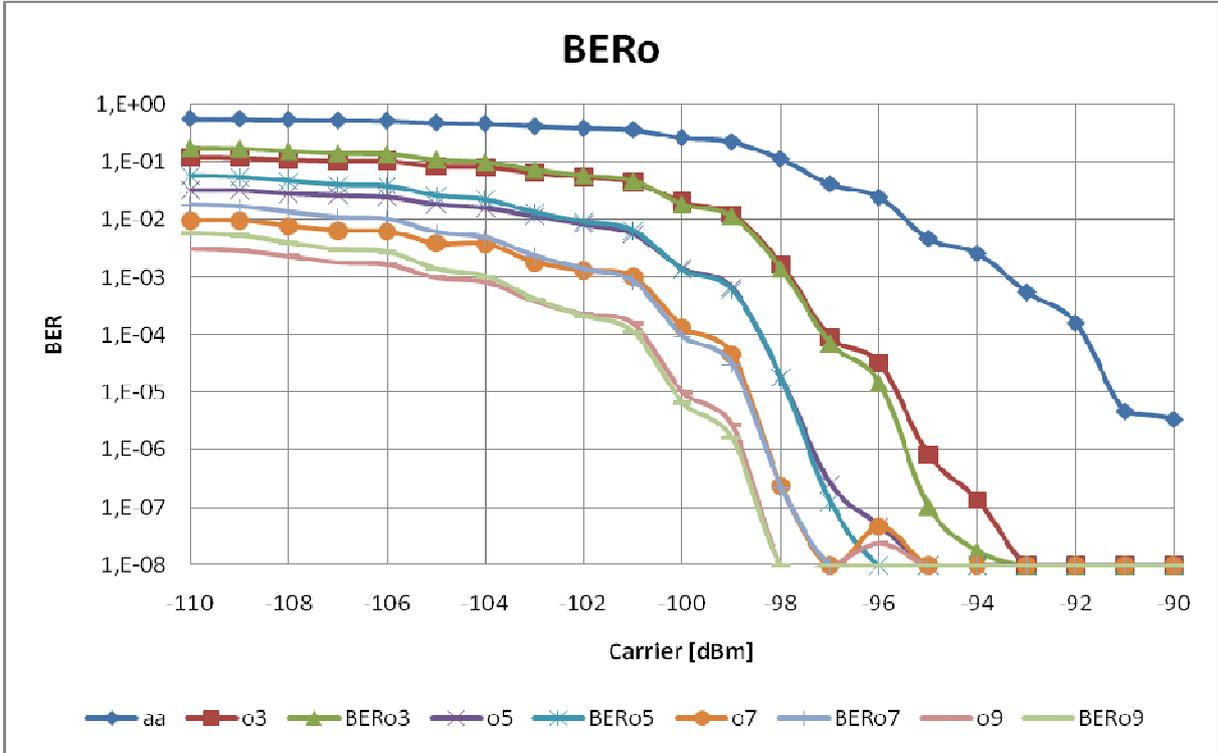
**Fig 8. Comparison of the optimal algorithm improving radio link quality depending on the number of receivers.**
