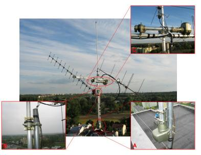
Figure 7. RC\_FNQ rotor (A - azimuth rotator, B - azimuth support bearing, C - elevation rotator with support bearing)
