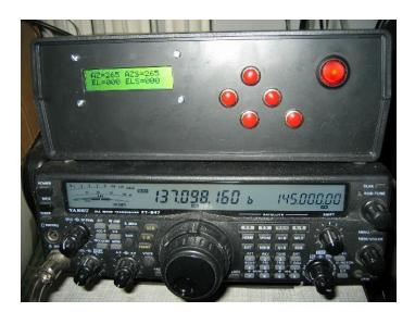
Figure 5. FNQ\_RC rotator controller on top of the Yaesu FT-847 satellite transceiver
