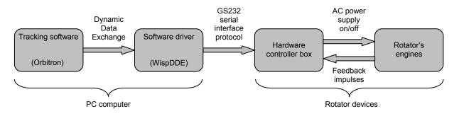
Figure 14. Data flow order in the antenna positioning system
