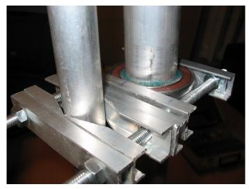
Figure 8. The support bearing for the rotator constructed by SP7DPT
