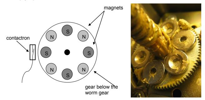
Figure 10. Rotation encoder for rotator
