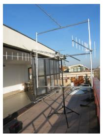
Figure 4. Left: stand "T" for manual satellite tracking, right: stand for manual tracking for YES2 mission
