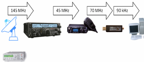
Figure 3. Structure of measurement system used for precise frequency estimation of PW-Sat.
