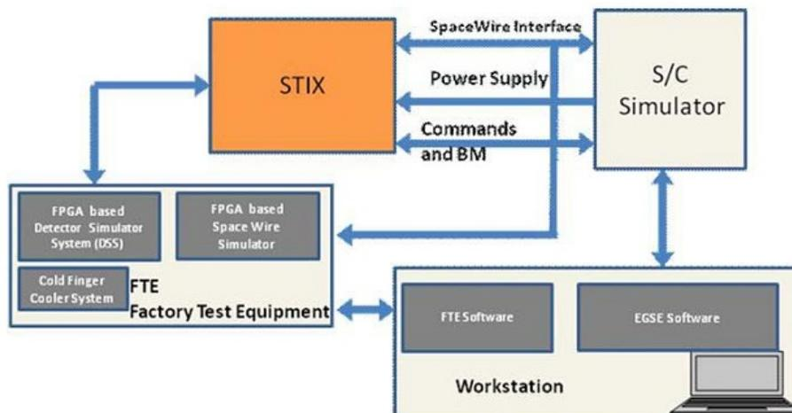
Figure 14. EGSE block schematics.
