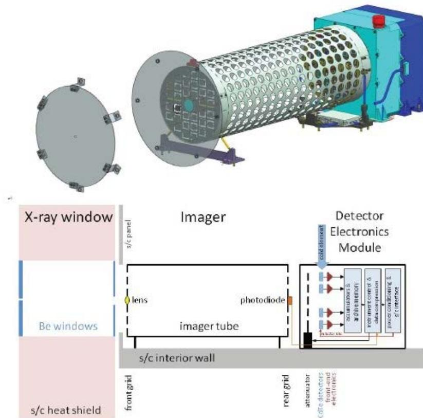
Figure 1. *Top*: The STIX instrument is made up of three mechanically-separate sections: the X-ray windows; the Imager with widely separated grids and aspect system; and the Detector/Electronics Module containing CdTe detectors and electronics. *Bottom*: Functional block diagram of the STIX instrument.
