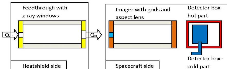
Figure 2. The scheme of the STIX instrument thermal design.  $Q_{sol}$  is the solar heat flux equal to 17.6 kW/m<sup>2</sup> at 0.28 AU,  $Q_{fi}$  is the heat flux between rear X-ray window and the Imager.
