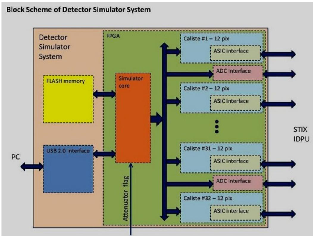
Figure 15. EGSE Detector Simulator internal block scheme.
