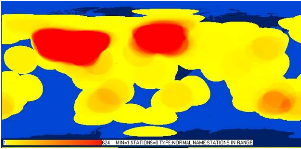
Fig 3. The number of ground stations in the range of a satellite.
