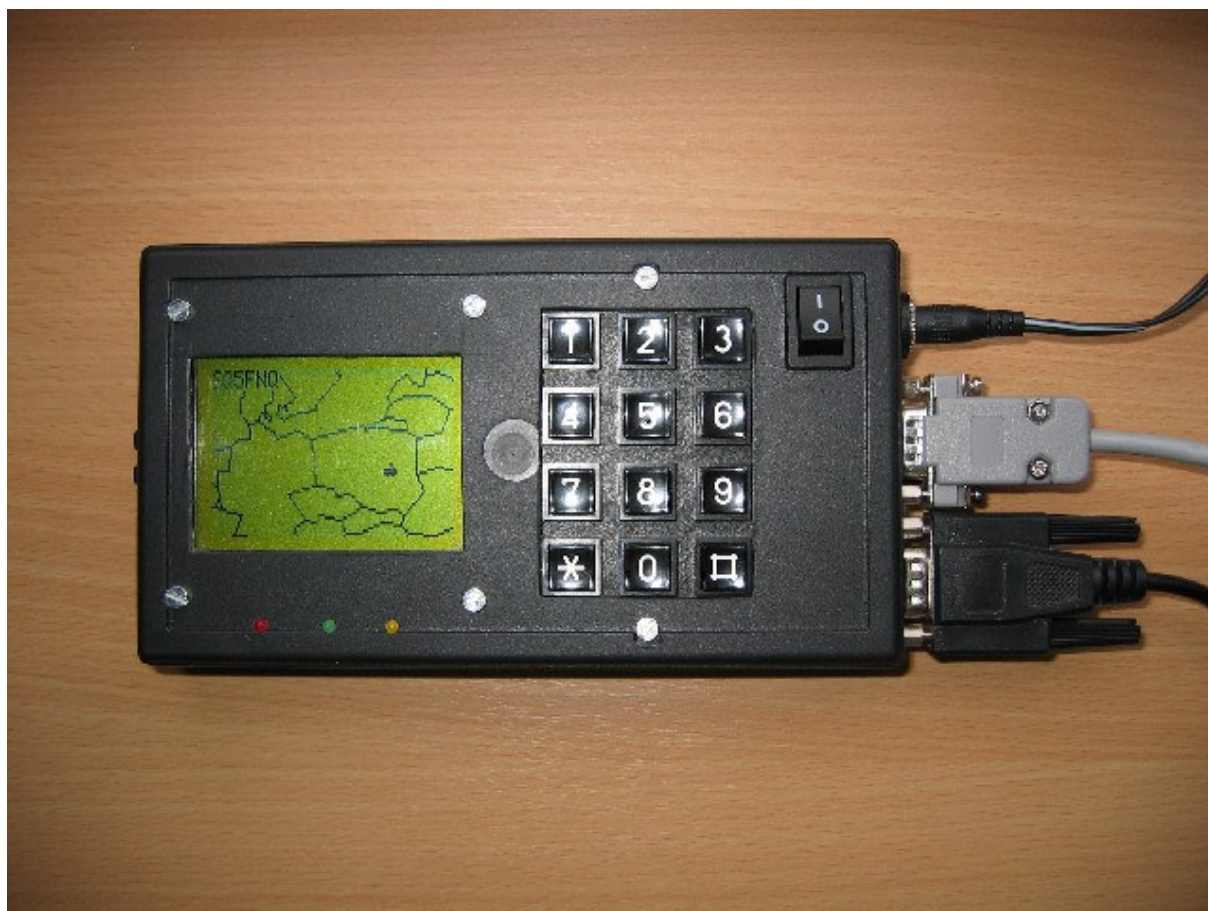
Rys. 25. Terminal APRS FOA-PACK.
