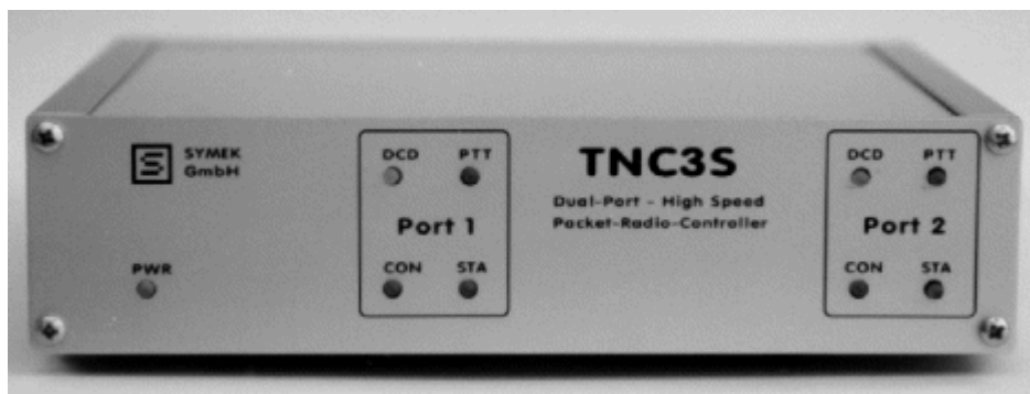
Rys. 18. Modem Packet Radio TNC3.
