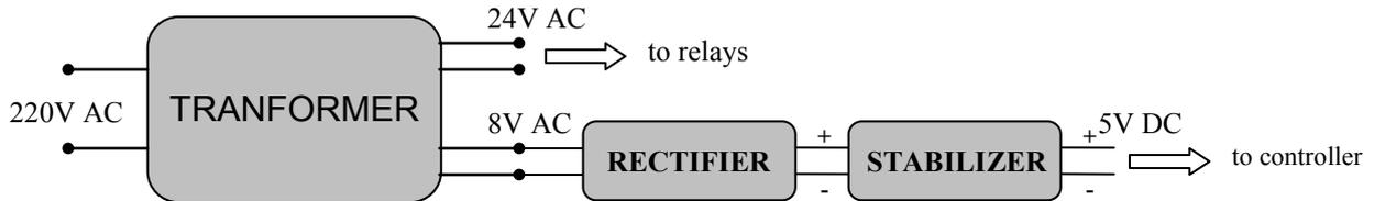
Figure 12. Block diagram of power supply
