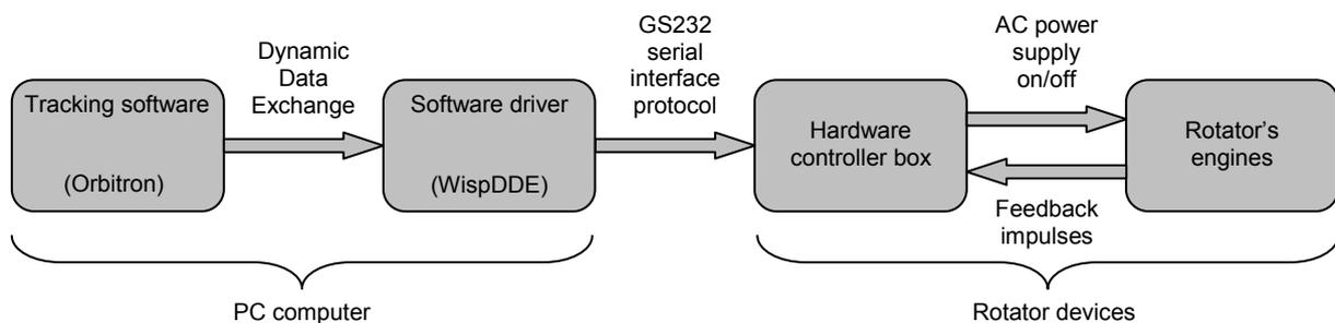
Figure 14. Data flow order in the antenna positioning system
