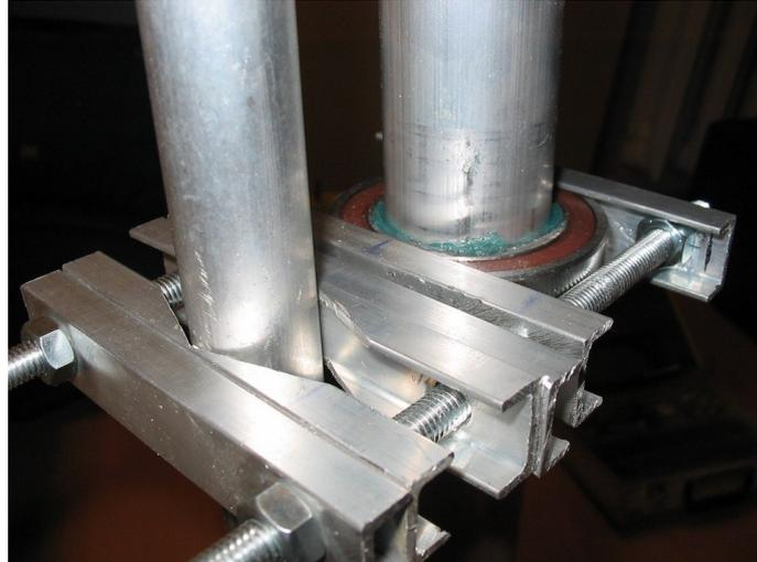
Figure 8. The support bearing for the rotator constructed by SP7DPT
