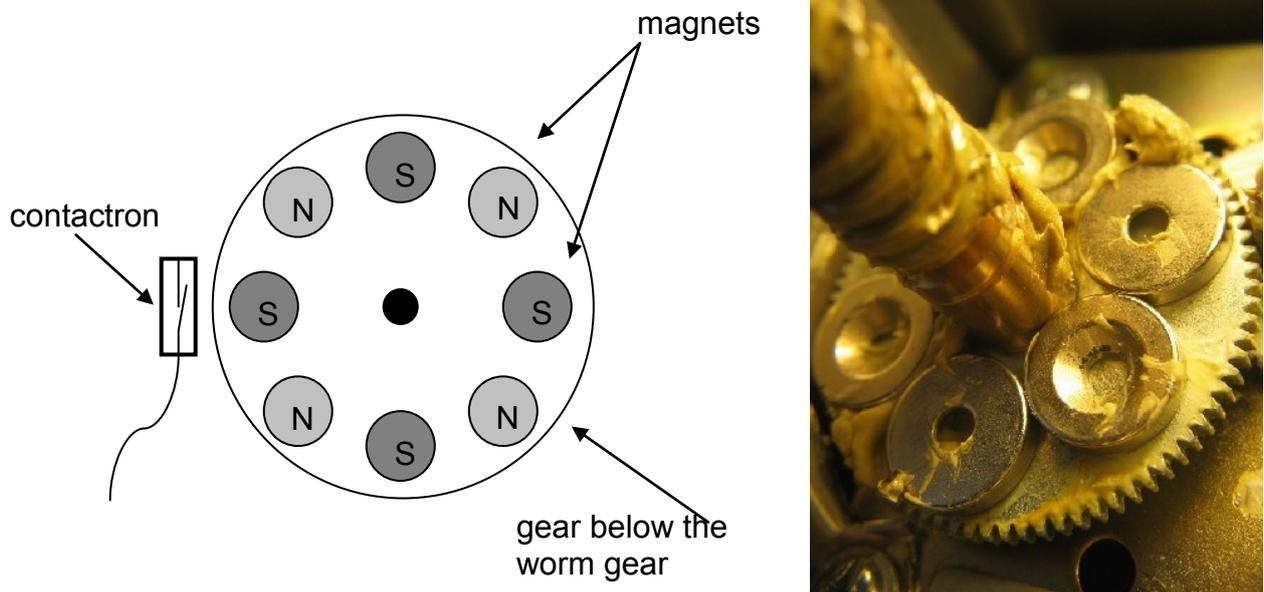
Figure 10. Rotation encoder for rotator
