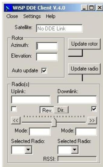
Figure 15. WiSP DDE Client software main interface
