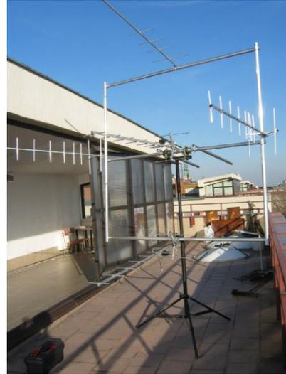
Figure 4. Left: stand "T" for manual satellite tracking, right: stand for manual tracking for YES2 mission
