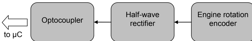
Figure 11. Block diagram of rotation encoder circuitry
